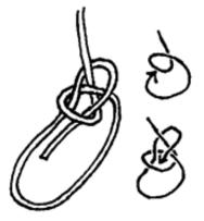
An extremely sturdy, and therefore safe, fixed loop. Used by emergency personnel to loop around a victim's body, under their armpits, for rescue operations. If properly tied, it will not grow or shrink under a load.
